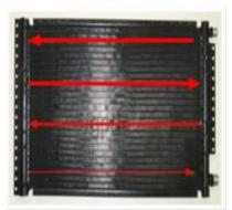
This is done by making the refrigerant change direction by 180° at the end on the side rails by placing a plug inside the rail at intervals, forcing the refrigerant change directions. The more plugs, the more times the refrigerant changes direction. In most condensers the refrigerant makes three to four "passes" through the condenser.
