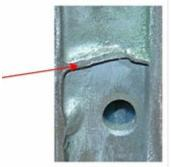
Parallel flow condensers don't have a large hollow tuve that the refrigerant flows through, but a series of verysmall tubes close together in a row with the internal diameter about the size of a pin head. This helps to improve the surface area of the condenser and increase its cooling capacity.
