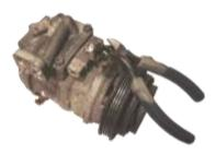
2. Cut connector from compressor. \* Make sure you have enough wire to make your electrical connection. DO NOT CUT NEXT TO COIL  $\stackrel{*}{\sim}$
