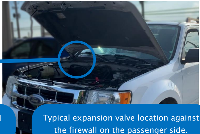
Expansion valve is in a vertical position in most vehicles.
