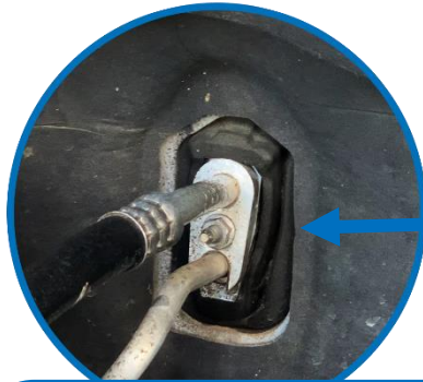
Expansion valve is in a vertical position in most vehicles.
