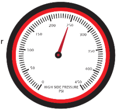
Overcharged or air blocked in the condenser
