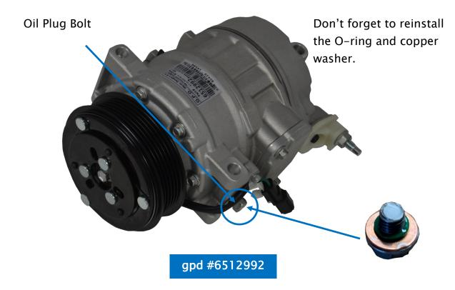
Refer to Tech Tip #44 for help on replacing the manifold from your old compressor.
