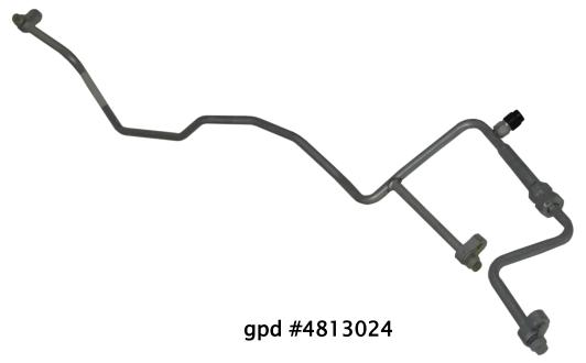
Liquid hose lines are typically made of aluminum and are designed with a lot of bends depending on the application. To improve durability, gpd has designed liquid hose lines made of steel for some applications. For the applications listed in this Tech Tip, gpd's steel design is a more durable and reliable replacement option than its aluminum counterpart.
