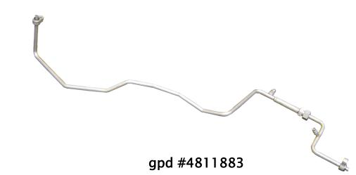
Liquid hose lines are typically made of aluminum and are designed with a lot of bends depending on the application. To improve durability, gpd has designed liquid hose lines made of steel for some applications. For the applications listed in this Tech Tip, gpd's steel design is a more durable and reliable replacement option than its aluminum counterpart.
