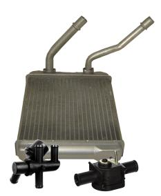
Some vehicles have "rear air", a rear air conditioning system. Vehicles with rear air have a second HVAC unit that includes an evaporator, blower motor, heater core, actuators, and rear expansion device. The compressor in the front system pumps refrigerant through a series of lines to the rear system as does the engine with coolant for the rear heater core. Failures in either system may cause damage to both.
